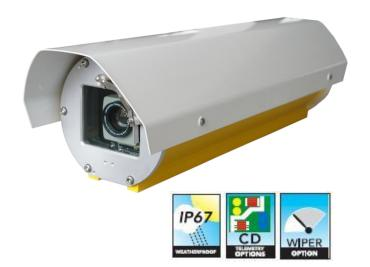
FBH01C flameproof camera housing is made by die-casting aluminum. There are two length available, FBH01C-30 and FBH01C-40. Power options include 110-230VAC and 12-24VAC/DC. There are four M20 thread holes in the rear cap and two ATEX certificated cable glands are supplied as standard. All holes are fitted with explosion proof stopping plug. The plug can be removed only if there is cable gland or tube to replace. Customer can choose camera and lens by themselves and fitted and tested in factory.
